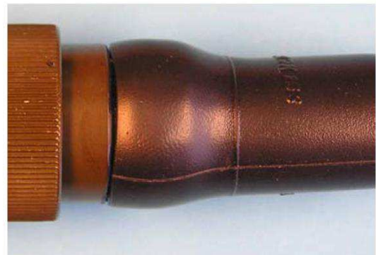
Adaptor body shall be free of excess adhesive
