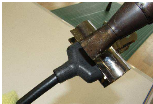
Figure 4 Apply heat towards 'J' end with 'H' end clamped
