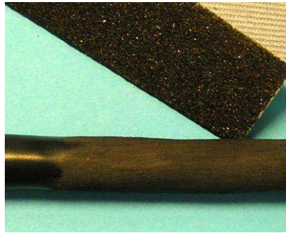
Figure 1 Degreased and abraded cable jacket
