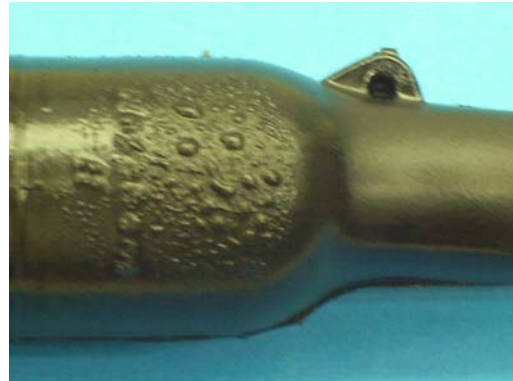
NOT ACCEPTABLE Scorch Marks
