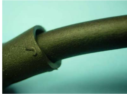
NOT ACCEPTABLE Under Recovered
