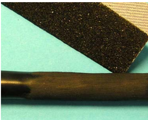
Cable Jacket Abrasion
