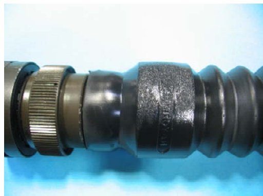
NOT ACCEPTABLE Scorch Marks
