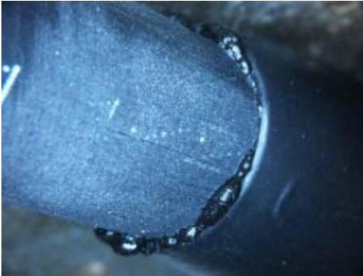
ACCEPTABLE 360° flow of adhesive
