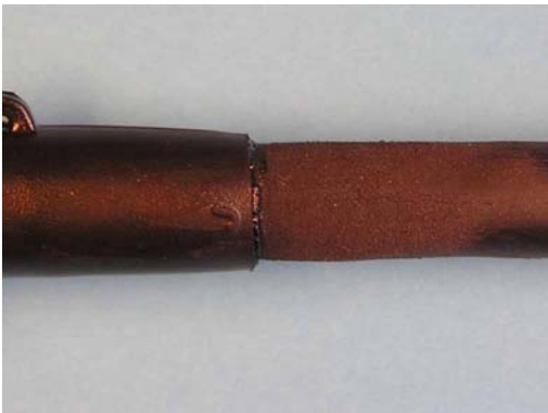
ACCEPTABLE 360° flow of adhesive
