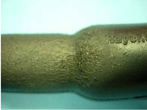
NOT ACCEPTABLE Scorch marks
