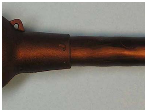
NOT ACCEPTABLE No evidence of adhesive flow
