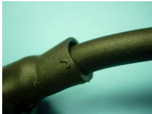
NOT ACCEPTABLE Under Recovered
