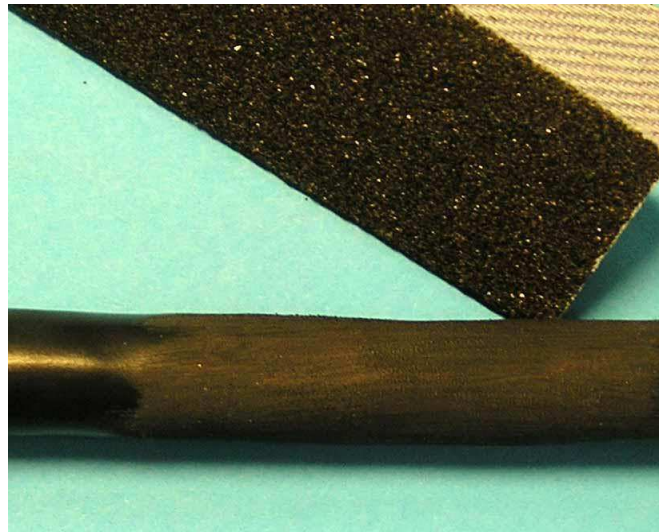
Figure 1 Degreased and abraded cable jacket
