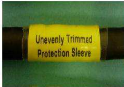
NOT ACCEPTABLE Unevenly Trimmed Tubing
