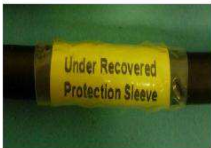
NOT ACCEPTABLE Insufficient Heat. Protection Sleeve Under Recovered
