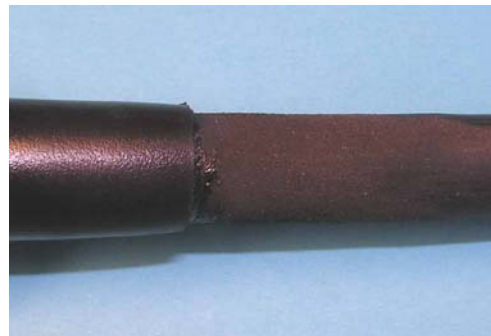
NOT ACCEPTABLE insufficient adhesive flow S1030, /180
