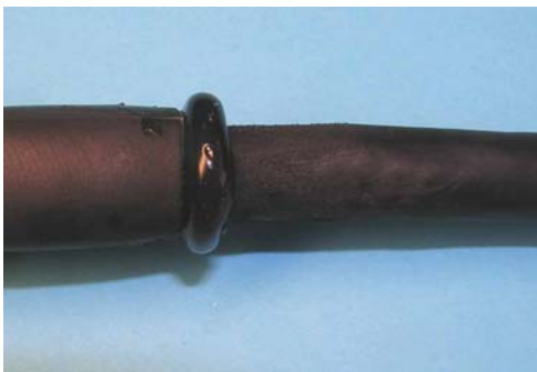
NOT ACCEPTABLE Excess adhesive flow S1030, /180
