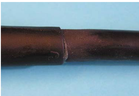
NOT ACCEPTABLE Insufficient adhesive flow S1048, /86, S1017, /42
