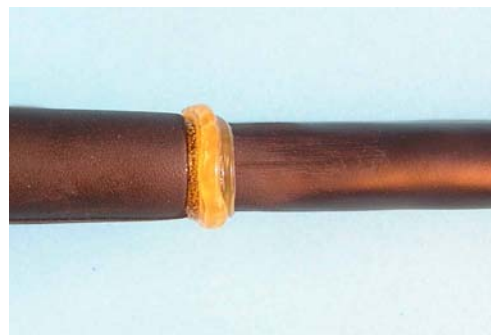
NOT ACCEPTABLE Excess adhesive flow S1048, /86, S1017, /42
