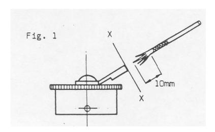
To ensure the best possible bond between the SCL tubing and the protection cover, degrease the protection cover where the SCL tubing will recover onto the tag with isopropyl alcohol or isopropanol (IPA) impregnated tissue wipe.
