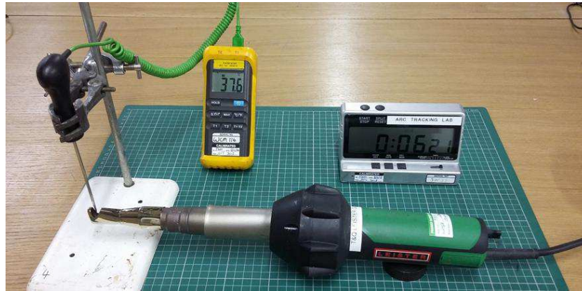
Figure 1 Hot air gun validation test setup
