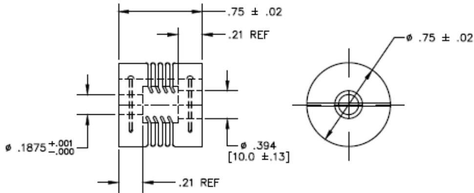
Figure 1: Coupling Adapter (Dimensions in inch [mm])
