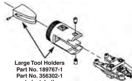
Platform Die Set Adapter Part No. 679992-1
