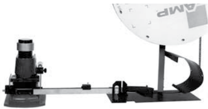
Manual Bench Tool with Applicator and Tape Feed Track
