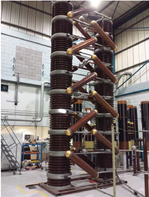
MARX impulse generator 1.6 MV
