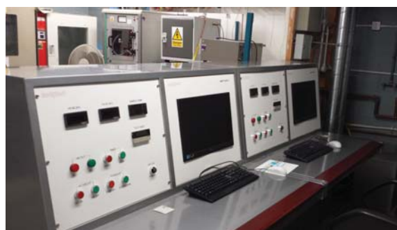
MOV ageing test system with variable frequency AC and DC test voltage and computer control data logger
