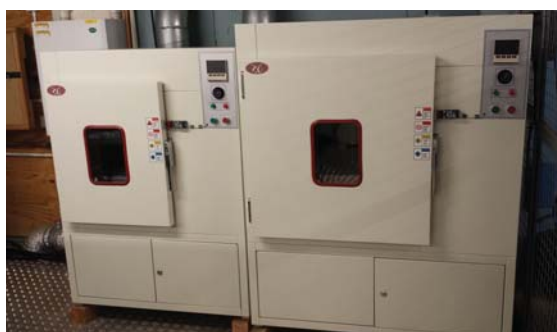
MOV ageing test system with variable frequency AC and DC test voltage and computer control data logger
