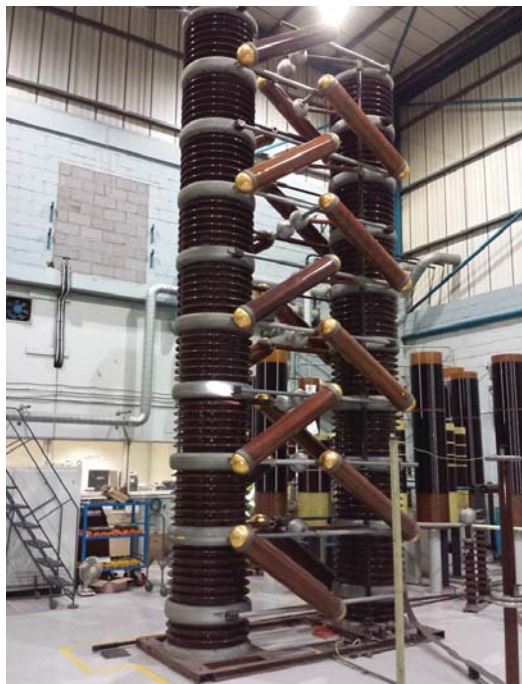
MARX impulse generator 1.6 MV
