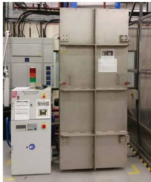
HV surge arrester helium leak test chamber for routine testing
