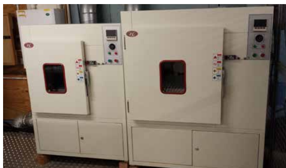
HV varistor block ageing test system with AC and DC supply
