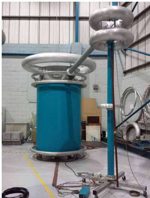
500 kV power transformer with PD testing
