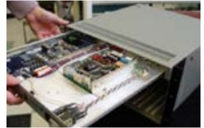
Figure 17: Inserting the front pull-out tray
