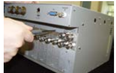
Figure 2: Remove sheet metal screws
