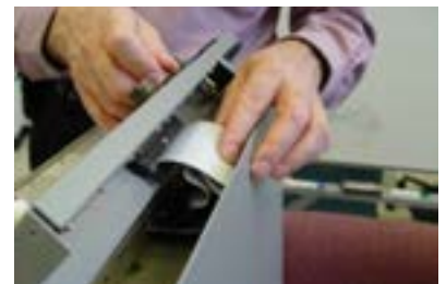
Figure 14: Folding the ribbon cable
