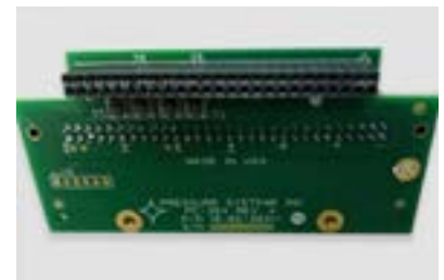
Figure 8: Backplane adapter board (PC364)
