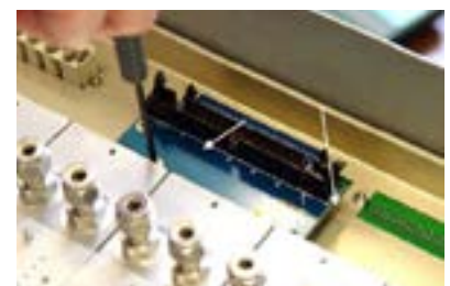
Figure 11: Attaching the backplane adapter board (PC364)
