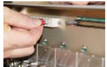
Figure 4: Removing wires from controller and switch assembly
