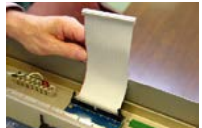
Figure 13: Connecting 60-pin ribbon cable to adapter board
