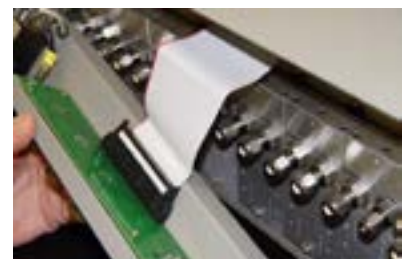
Figure 5: Ribbon cable connection from rack to controller and switch assembly
