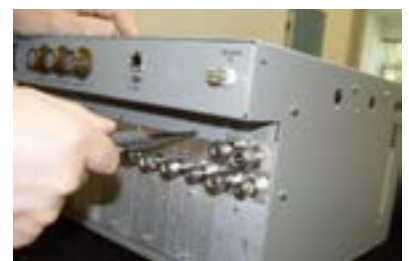
Figure 16: Inserting the rear panel sheet metal screws.
