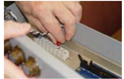
Figure 12: Attaching spade connectors
