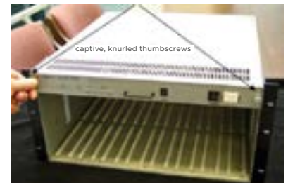
Figure 6: Removing front pull-out tray
