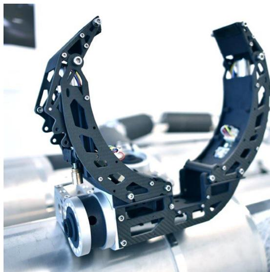
Fig 5: Monkeybot for robotic sensor installation
