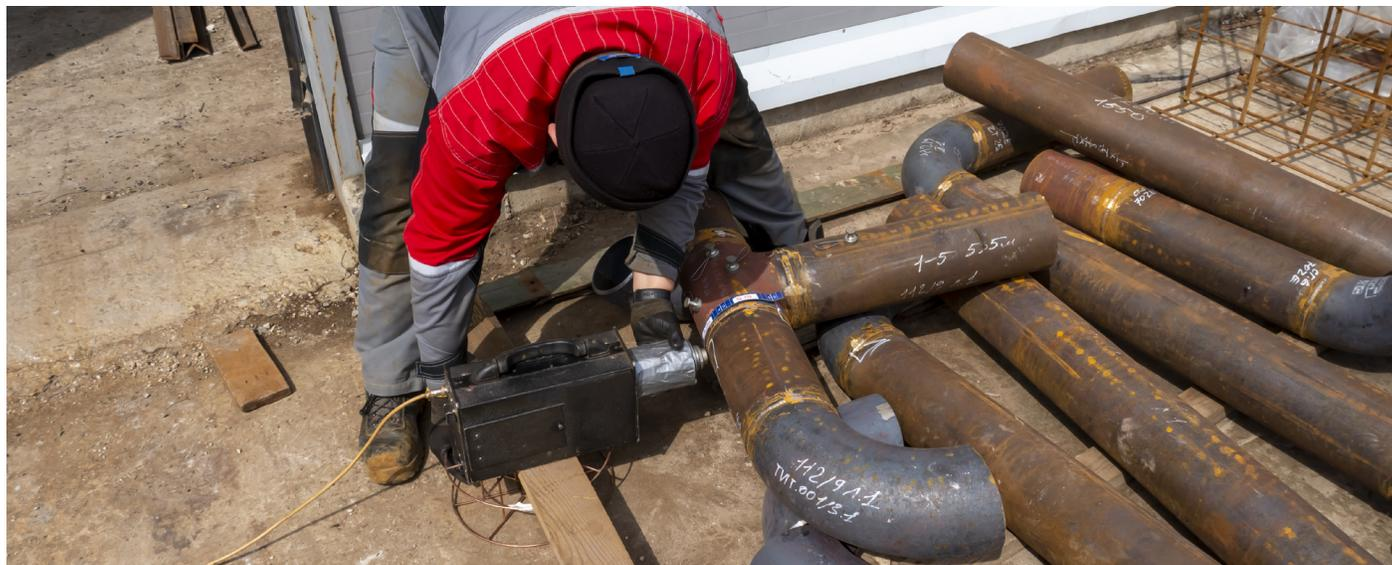
Fig 3. A specialist installing an X-ray device for non-destructive evaluation of welded joints.
